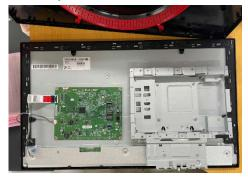
LCD module(together with their casing) is only left after all other parts like electronic units and casing have been removed.
