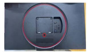
Overturn the set and disassemble the latches of three edges
