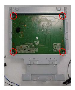
Disassemble the screw and Main PCB
