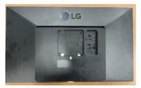
Re-overturn the set and disaaemble screw 4EA+4EA and disassemble the PCB
