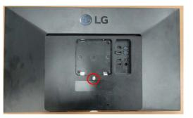
Overturn the set use jig to disassemble backcover
