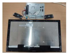
LGD module(together with their casing) is only left after all other parts like electronic units and casing have been removed.
