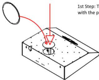
1st Step: The exhaust hole will be closed with the plastic cover.
