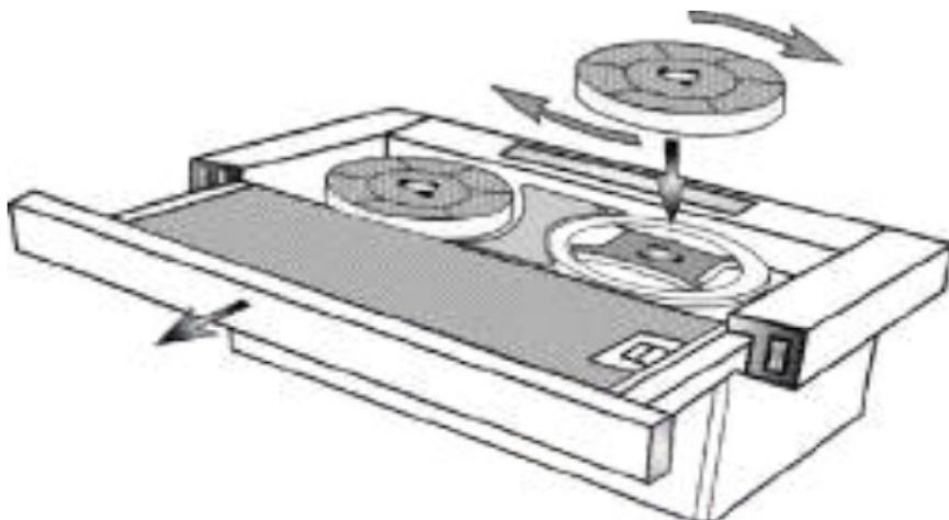
To maintain odor insulation levels, regular care of the filter is necessary. The active carbon filter should be replaced every 4 months.
