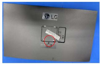
Overturn the set and disassemble the latches of three edges
